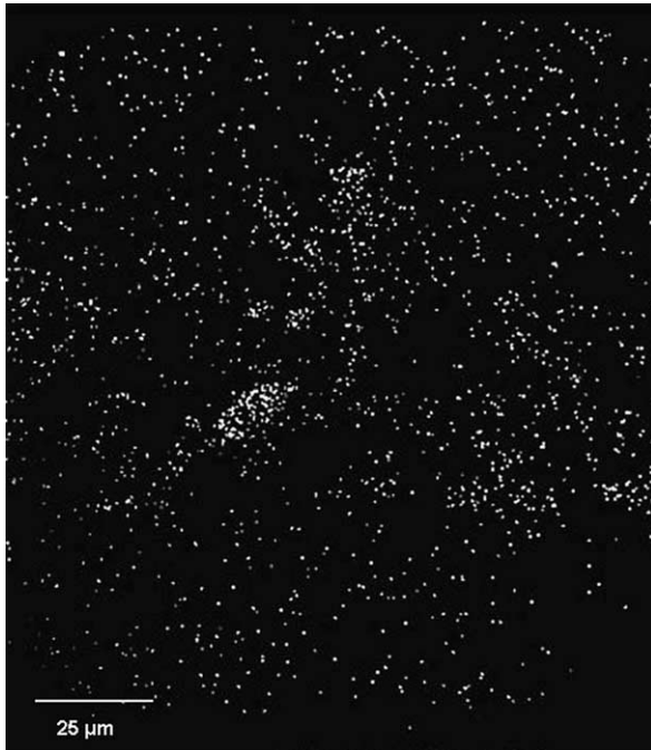
Fig. 4. X-ray dot mapping of Tc in area as shown in Fig. 2.
